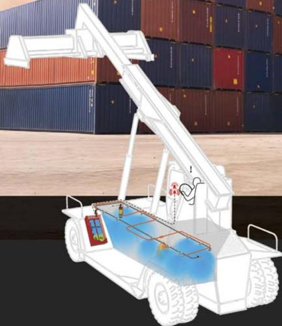
The Fogmaker fire suppression system is tailor-made for each type of material handling equipment. High-pressure water mist chokes fires quickly and cools the area to prevent reignition. Fogmaker's system is automatic, independent of electricity, and always ready!
